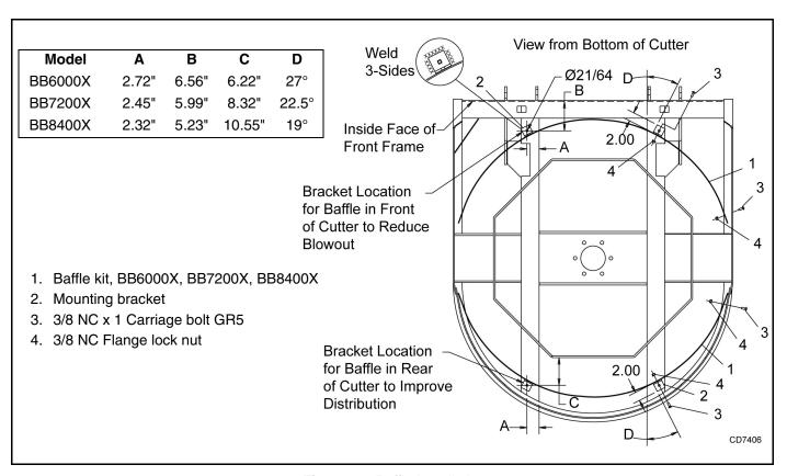
Figure 34. Baffle Installation
